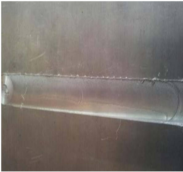
Fig: 2.2 welding plate on 710 rpm
